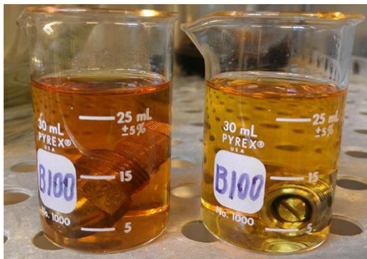
Figure 4-1 High temperature metals exposure test, B-100. Appearance of the B-100 sample with a brass nozzle (left) and stainless-steel nozzle (right) after 1 week at 175 F.
