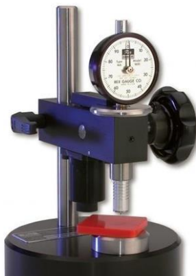
Figure 1-2. Type M Durometer used for hardness measurements of the nitrile samples before and after exposure to fuels.
