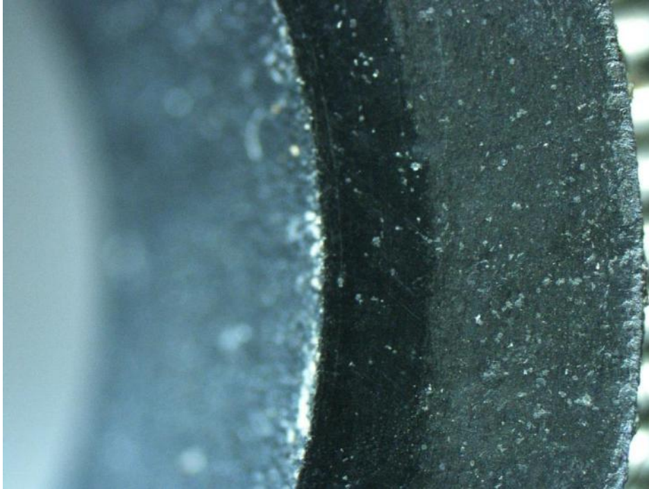
Figure 2-6 Image of the sealing edge of a new oil burner shaft seal.
