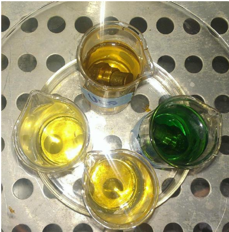
Figure 4-3 Samples of ULS (B0). Impact of extremely elevated acid number and a nozzle over one weekend at room temperature.
