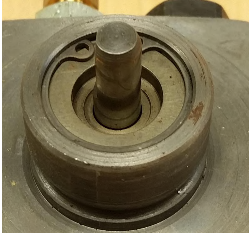
Figure 2-2 Photo of pump with a carbon face seal after 11 months of testing with biodiesel.
