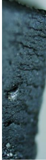
Figure 2-9 Image of the sealing edge of a shaft seal from one of the pumps in the Penn State long term test. This pump operated with a B0 blend.
