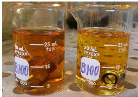
Figure 1 Fuel nozzles exposed to B20 blends for 4 weeks at 175 F. Left - brass nozzle, Right - stainless steel nozzle.
