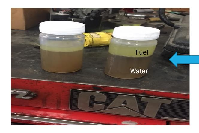
Sample from Class 8 truck fuel filter water separator.
